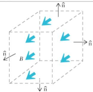
**Region of nonzero magnetic field moving to right, at speed  $v$ .**
