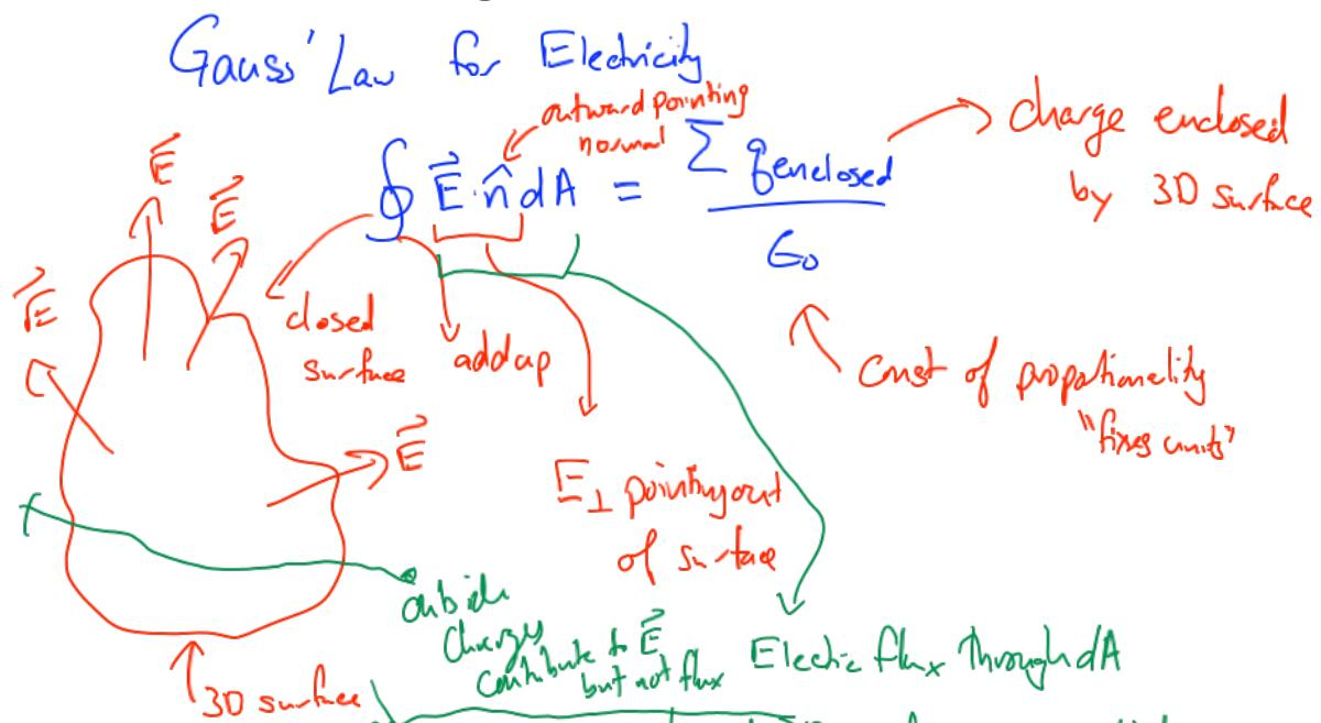
Total electric flux through a closed 3D surface is proportional to  $(1/\epsilon_0)$  the total electric charge inside that surface.
